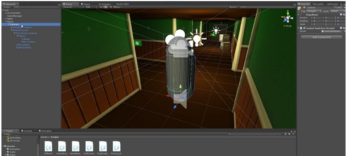
Figure 5-10. Attaching a ControlSwitcher script to the Controls object. This script will deactivate the redundant First Person Controller on scene start-up
