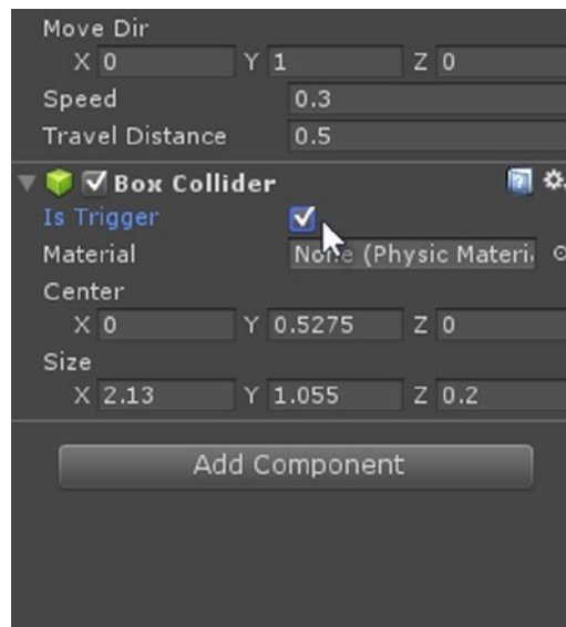
Figure 4-11. Enable “Is Trigger” to receive collision notifications in the script when collisions happen
