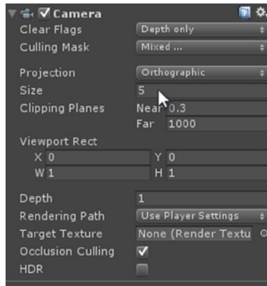
Figure 6-13. The size member of orthographic cameras controls the size of graphical elements on-screen
