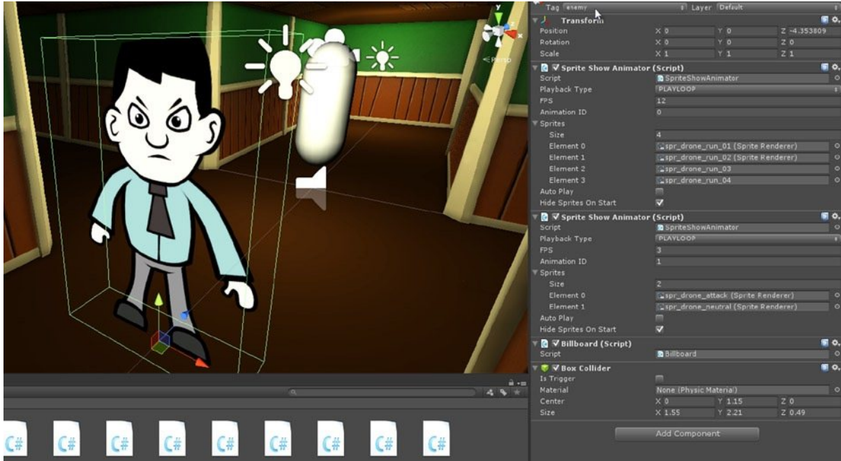
Figure 7-7. Configuring the Drone enemy with a Billboard component and a BoxCollider component
