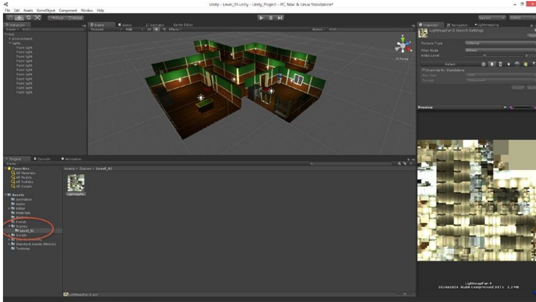
Figure 2-33. Generated lightmaps are added to the project like a regular texture and are accessible via the Project panel
